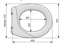
Opening angle: 115°. Load capacity: up to 150 kg Weight without hinge: approx. 2 kg
